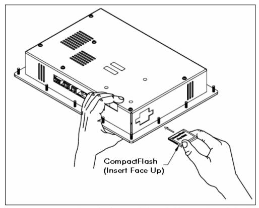
**Note:** Do not remove or insert the CompactFlash card while power is applied to the unit. Refer to the "Front Panel LEDs" section of this document for more information.
