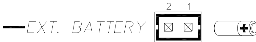
Figure 16 External battery connector for GF_VEDO HL terminals
