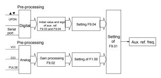
Fig. 5-60 Auxiliary reference frequency selector
