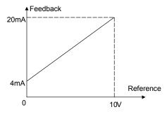
Fig. 5-32 Reference and feedback
