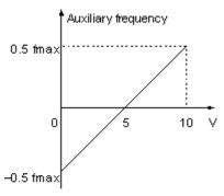
fmax — frequency corresponding to Max analog value (F1.07 or F1.11)
