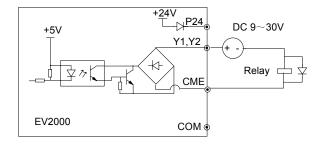
Fig. 3-29 Wire connections 2 of multi-function output terminal
