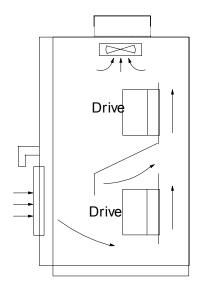
Fig. 3-3 Installation of several drives
