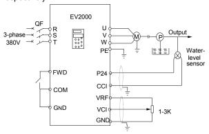
Fig. 5-29 Analog feedback control system with internal PI
