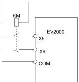
Fig. 5-41 Normally-open/close input
