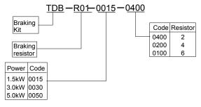
Fig. 2-7 Explanations of Model of braking resistor
