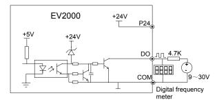
Fig. 3-31 Wiring 2 of output terminal DO
