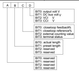
Fig. 5-53 Operating parameter 2 displayed by LED
