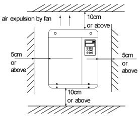
Fig. 3-1 Installation clearance (45kW or below)
