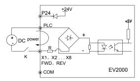
Fig. 3-23 Using an external supply
