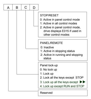
Fig. 5-64 Functions of keys and panel locking up function
