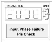
Fig. 4-5 Alarm displaying status
