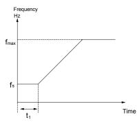
Fig. 5-12 Starting frequency and starting time
