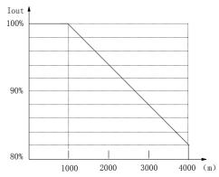
Fig. 1-3 Derating Drive's output current with altitude
