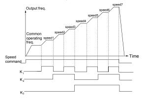
Fig. 5-39 Multi-step speed operation
