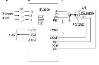
Fig. 5-30 Wiring of speed close-loop with PG
