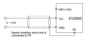
Fig. 3-14 Wiring terminal VCI
