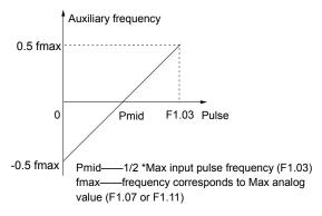
Fig. 5-62 PULSE-0.5×F1.03 as auxiliary ref. setting method
