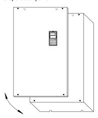
Fig. 3-6 Removing and mounting metal cover
