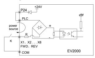
Fig. 3-22 Using internal 24V power supply
