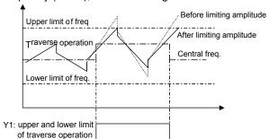
Fig. 5-46 Traverse operating amplitude control
