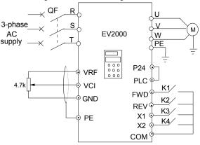
Fig. 5-58 Wiring of remote and local control
