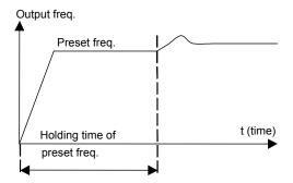
Fig. 5-36 Preset frequency of close-loop operation
