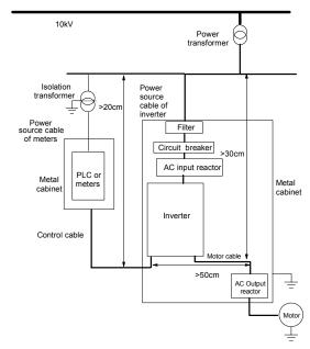
Fig. 3-44 Installation of the drive
