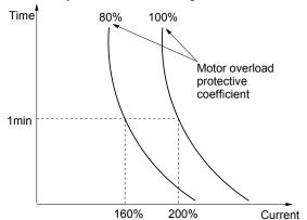
Fig. 5-71 Motor's overload protection coefficient
