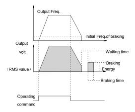
Fig. 5-16 Dec-to-stop + DC injection braking
