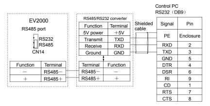
Fig. 3-18 RS485-(RS485/RS232)-RS232 communication cable
