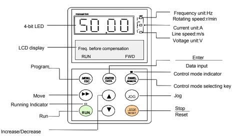
Fig. 4-2 Illustration of operation panel
