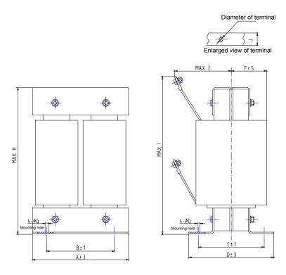
Fig. 2-3 Dimensions of DC reactor
