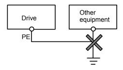
Fig. 3-39 Earthing diagram 3
