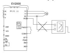
Fig. 7-2 Insulation test of motor
