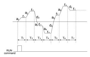
Fig. 5-24 Maintaining the frequency after single cycle
