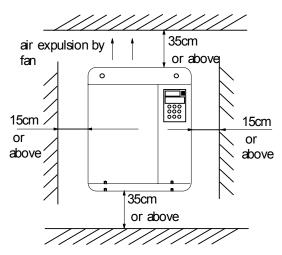
Fig. 3-2 Installation clearance(55kW or above)
