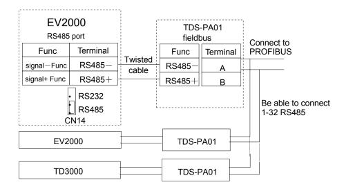
Fig. 3-20 Wire connections of RS485-(TDS-PA01)-PROFIBUS communication
