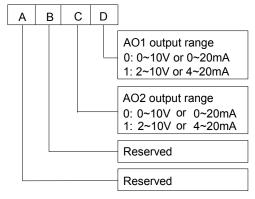
Fig. 5-49 analog output offset settings
