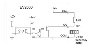
Fig. 3-30 Wiring 1 of output terminal DO
