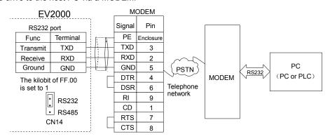
Fig. 3-19 Wiring of RS232-(MODEM-PSTN-MODEM)-RS232 communication
