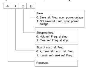
Fig. 5-63 Digital auxiliary reference frequency control
