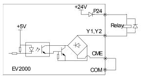
Fig. 3-28 Wire connections 1 of multi-function output terminal
