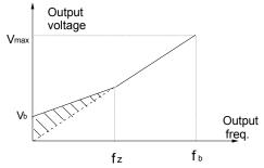
V<sub>b</sub>: Manual torque boost Vmax: Max output voltage
