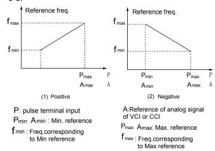
Fig. 5-8 Output frequency curve
