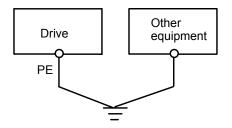
Fig. 3-38 Earthing diagram 2
