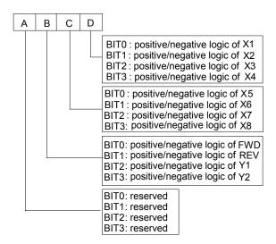
Fig. 5-51 terminal's positive and negative logic
