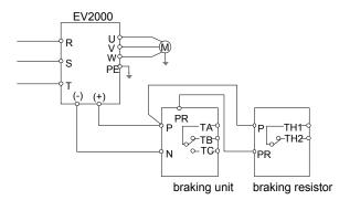
Fig. 2-10 Connecting the braking kit to the Drive
