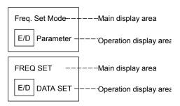
Fig. 2-5 LCD display interface
