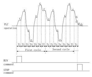
Fig. 5-25 Continuous operation of PLC
