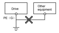
Fig. 3-40 Earthing diagram 4
