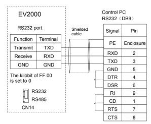
Fig. 3-17 RS232-RS232 communication cables
