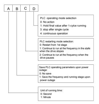
Fig. 5-22 Simple PLC operation mode
