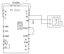
Fig. 7-1 Insulation test of drive
