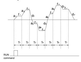
Fig. 5-23 Stopping mode after single cycle of PLC
