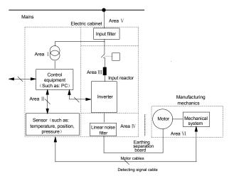
Fig. 3-43 Recommendation of Installation space
