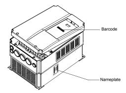
Fig. A-3 Locations of Nameplate and Barcode
