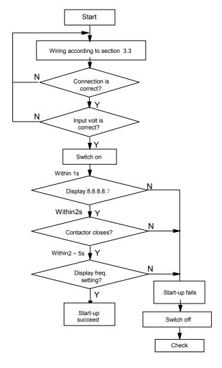
Fig. 4-8 Procedures of starting the drive for the first-time
