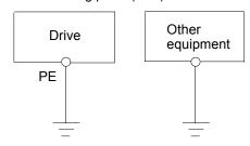
Fig. 3-37 Earthing diagram 1
