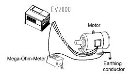
Fig. 1-1 Checking the insulation of motor
