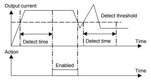
Fig. 5-74 Overload pre-alarm function
