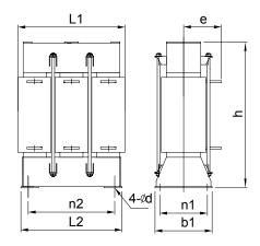
Fig. A-2 Outline of 3-PH AC input and output reactor (b)
