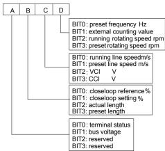
Fig. 5-55 Stopping parameters displayed by LED
