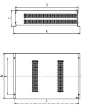
Fig. 2-9 Installation dimensions of braking resistor
