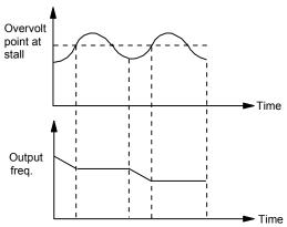
Fig. 5-72 Over-voltage at stall
