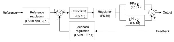
Fig. 5-31 PI block diagram
