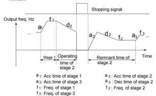
Fig. 5-27 PLC starting mode 2
