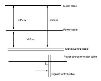
Fig. 3-34 Wire connections
