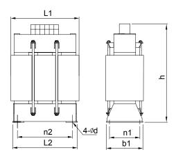
Fig. A-1 Outline of 3-PH AC input and output reactor (a)
