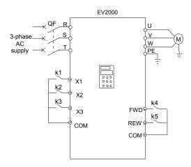
Fig. 5-40 Wiring for multi-speed operation
