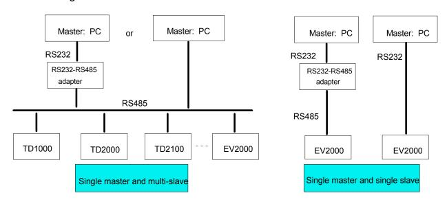
Fig. A-6 Networking diagram of drives
