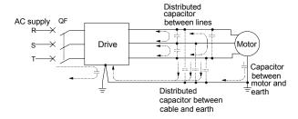
Fig. 3-42 Flowing path of leakage current
