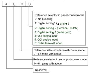
Fig. 5-56 Control mode is bundled to frequency selector
